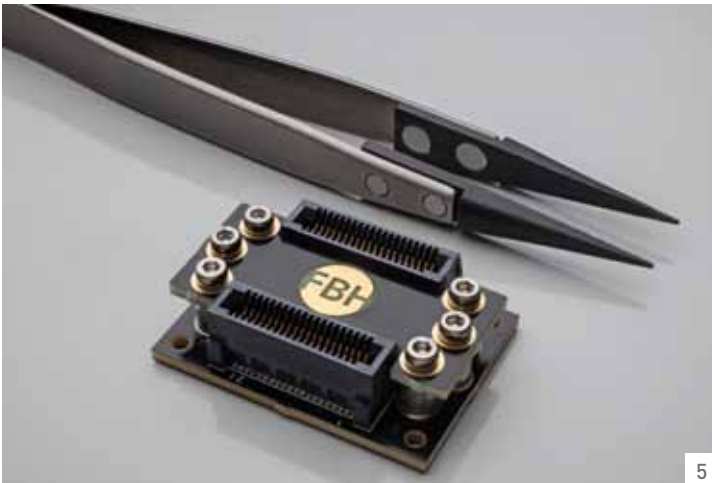
3 merging the best of two technology worlds – integrated InP-on-BiCMOS chip
